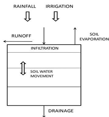
Fig. 1. Scheme of the soil water balance simulated by DSSAT
