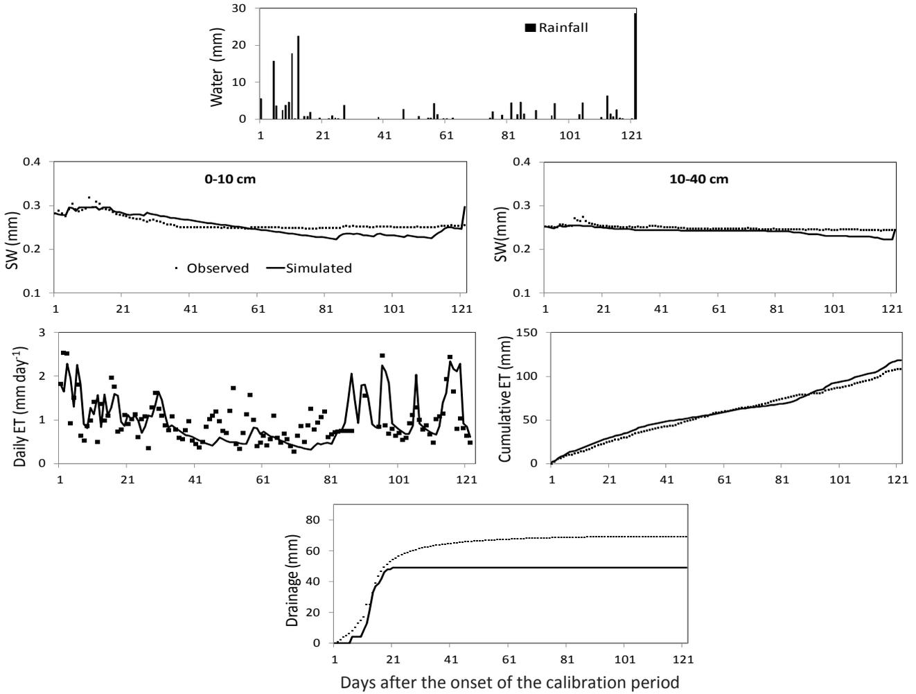
**Fig. 4.** Simulated and observed soil water balance components (soil water content, drainage and ET) during the second period (October 2012- February 2013) of the experiment
